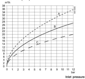
A) d = 8 mmNozzles B) d = 7 mmC) d = 6 mm
